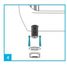
Secure the valve to the cistern using the plastic washer and nut. Do not over tighten.
