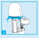
Turn the water supply on and off to clear any debris. Hold a cup over the top to prevent any splashing.
