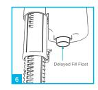
The valve comes with a delayed fill function which delays the filling of the cistern until 5 seconds (approx.) after the start of a flush
