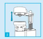
Lift the top assembly away from the valve holding the arm.
