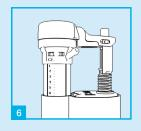
Refit top assembly complete with diaphragm and tun on water supply.
